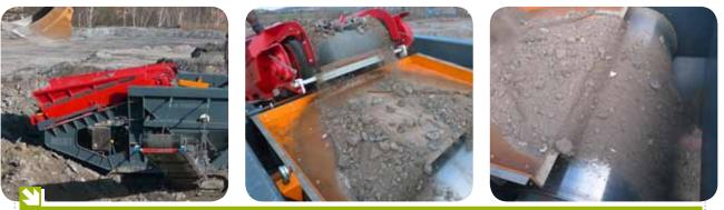
Compared with stationary plants, the mobile magnetic separator can easily be placed on the jobsite and follows the material. This allows a reduction of logistic costs and therefore an economic operation.
